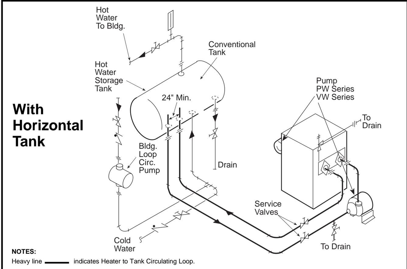
Figure 11 – Hot Water Supply System (Model VW & PW)
