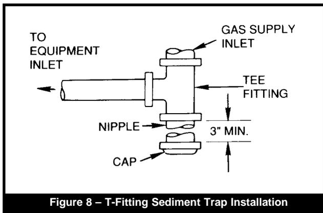
**Figure 8 – T-Fitting Sediment Trap Installation**
