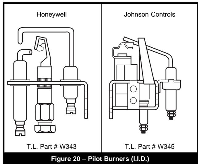
**Figure 20 – Pilot Burners (I.I.D.)**
