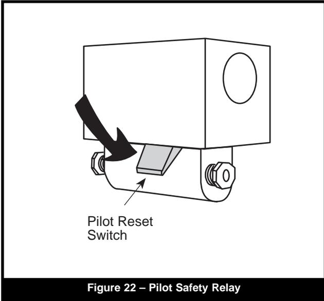
Figure 22 – Pilot Safety Relay
