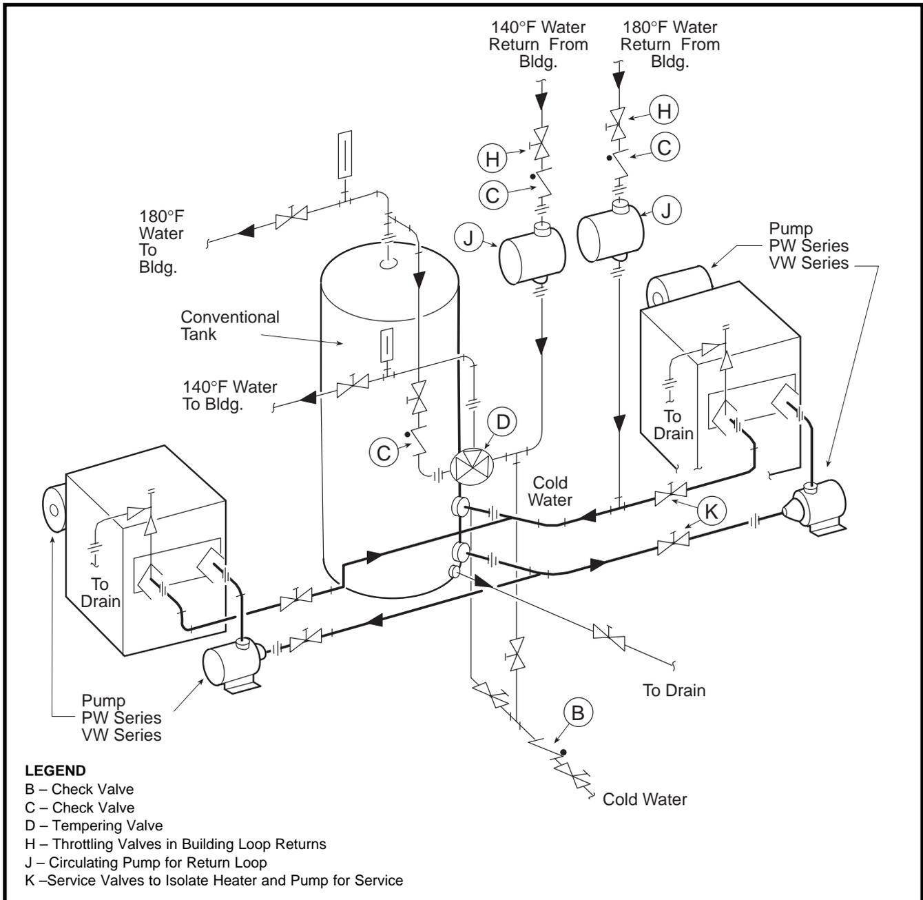
Figure 17 – Two-Temperature Hot Water Supply System with Vertical Tank for Models VW and PW Water Heaters
