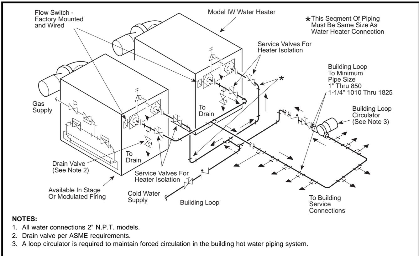
Figure 14 – Dual Installation Piping Diagram, Model IW
