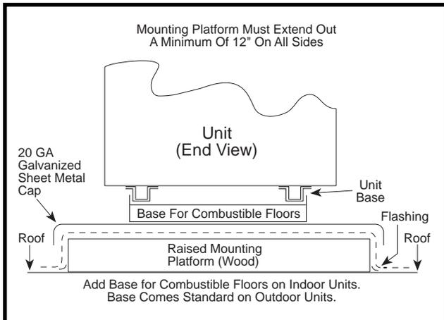
**Figure 3 – Typical Heater Installation with Base for Combustible Floors, Example B**
