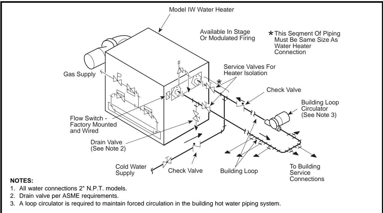
Figure 15 – Single Installation Piping Diagram, Model IW
