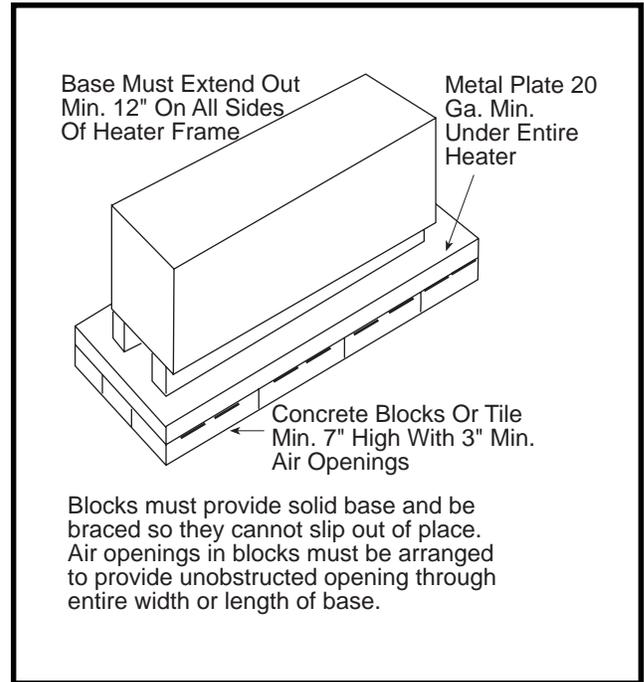
**Figure 5 – Installation on Concrete Blocks or Tile**
