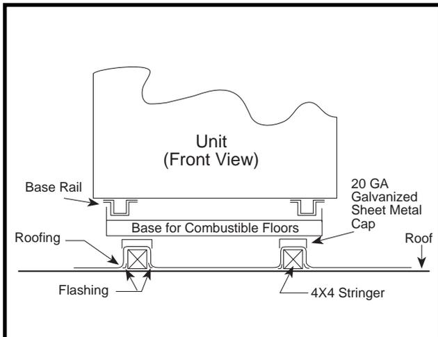
**Figure 4 – Typical Heater Installation with Base for Combustible Floors, Example C**
