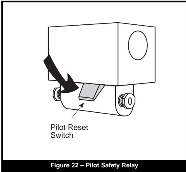
Figure 22 – Pilot Safety Relay
