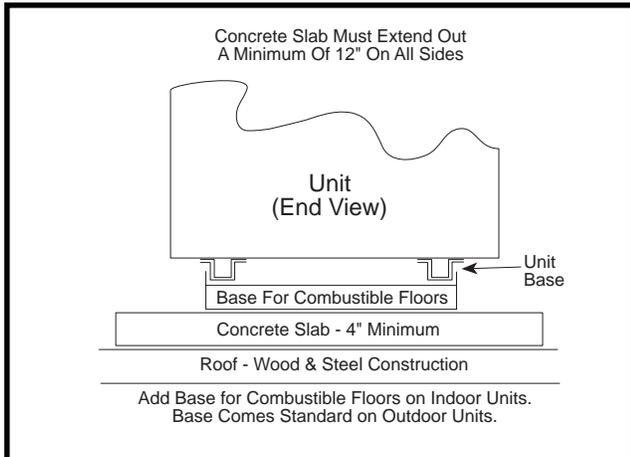
**Figure 2 – Typical Heater Installation with Base for Combustible Floors, Example A**
