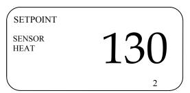
5. Press the **SELECT** button again. You will see the following display. The number displayed is the differential for stage 2. This is the number of degrees under the set point for stage 2 at which the steam system, or stage 2, is activated (i.e. steam solenoid opens). 5 is the standard and recommended setting. Use the arrow keys to set the desired number. Press **ENTER** when done.
