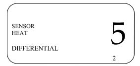
6. Press **SELECT**. You are now done! The basic display will show the sensor temperature. The 'STAGE ENERGIZED' will tell you what the control is doing. If you see '1', then the condensate system is on. If you see both '1' and '2', that means that both the condensate system and the steam system is on. If you see '2' on without '1', the control has not been wired correctly.
