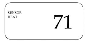
2. Press the **SELECT** button again. You will see the following display. The temperature displayed is the condensate set point. This is the maximum temperature of water you want. Press the up or down arrow keys under **SET** to set the set point to the desired value. In many applications this is 140°. The '1' displayed below the set point temperature tells you that this is for stage 1, or for the condensate stage. Use the arrow keys to set the desired temperature. Press **ENTER** when done.
