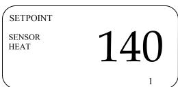
3. Press the SELECT button again. You will see the following display. The number displayed is the differential. This is the number of degrees under the set point at which the condensate system, or stage 1, is activated (i.e. the bypass solenoid closes, the condensate solenoid opens, and condensate enters the lower heat exchanger). 5 is the standard and recommended setting. Use the arrow keys to set the desired number. Press **ENTER** when done.
