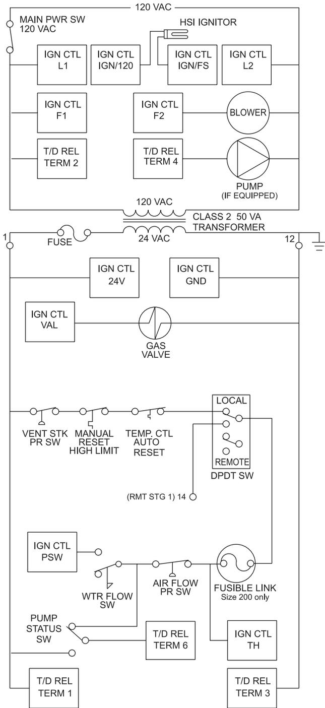
Figure 17. Logic Diagram, ON/OFF Boiler or Water Heater.
