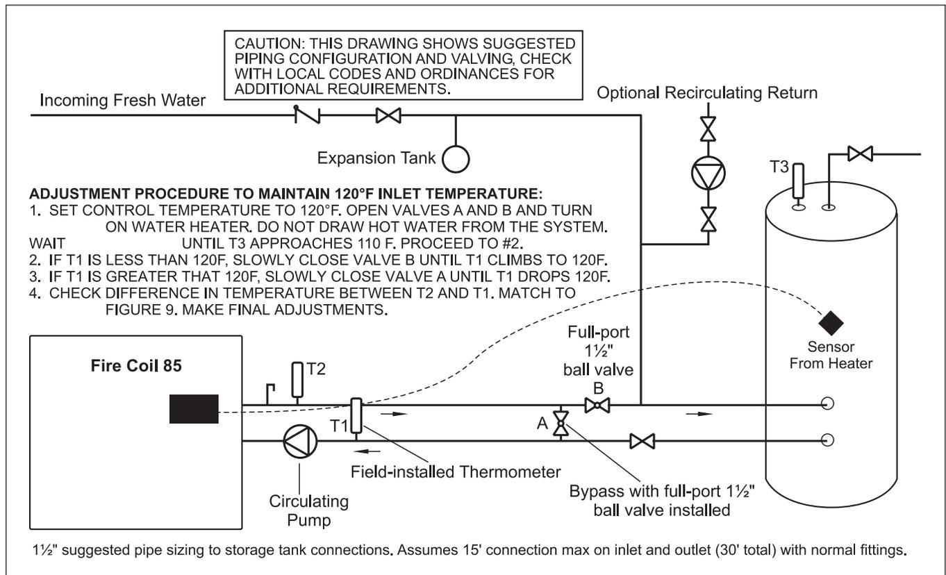
**Supplemental Drawing - Low Temperature Stored Hot Water Applications.**
