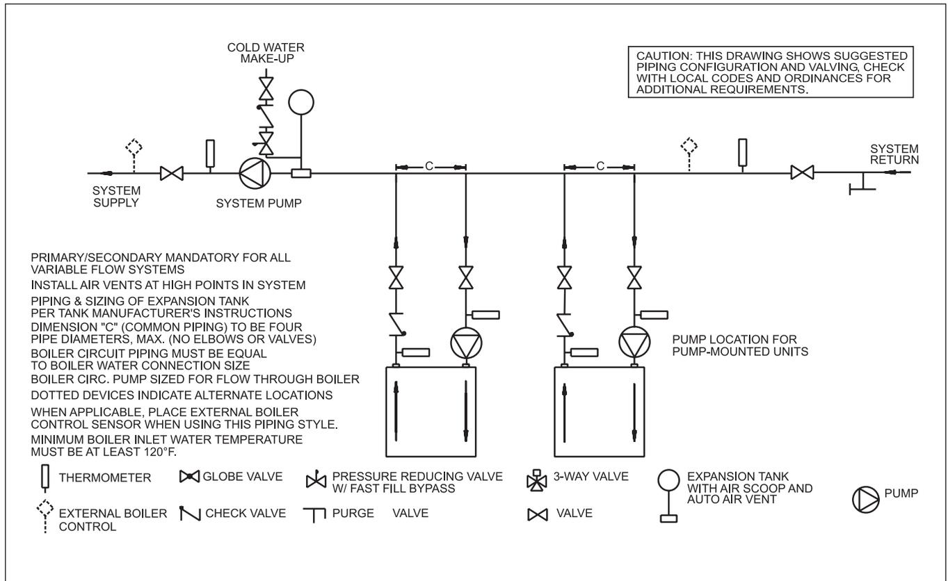
Figure 4. Hydronic Piping — Multiple Boilers, Primary Secondary System.
