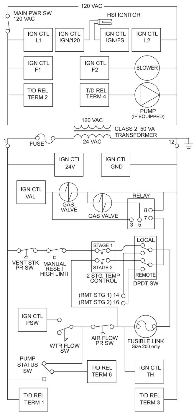
Figure 18. Logic Diagram, 2-STAGE Boiler or Water Heater.
