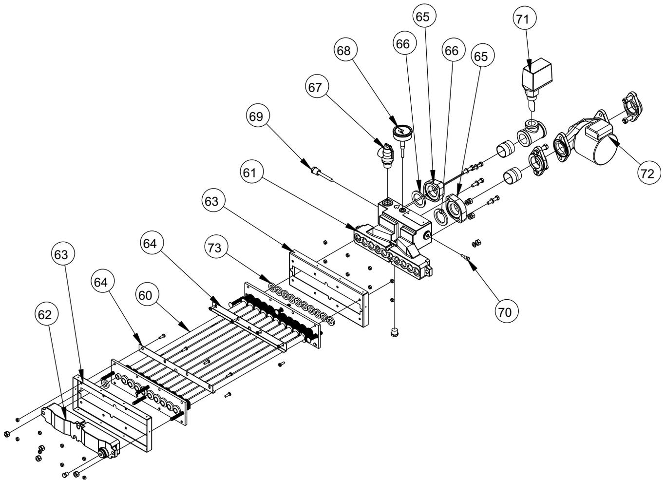
Figure 22. Heat Exchanger Components.
