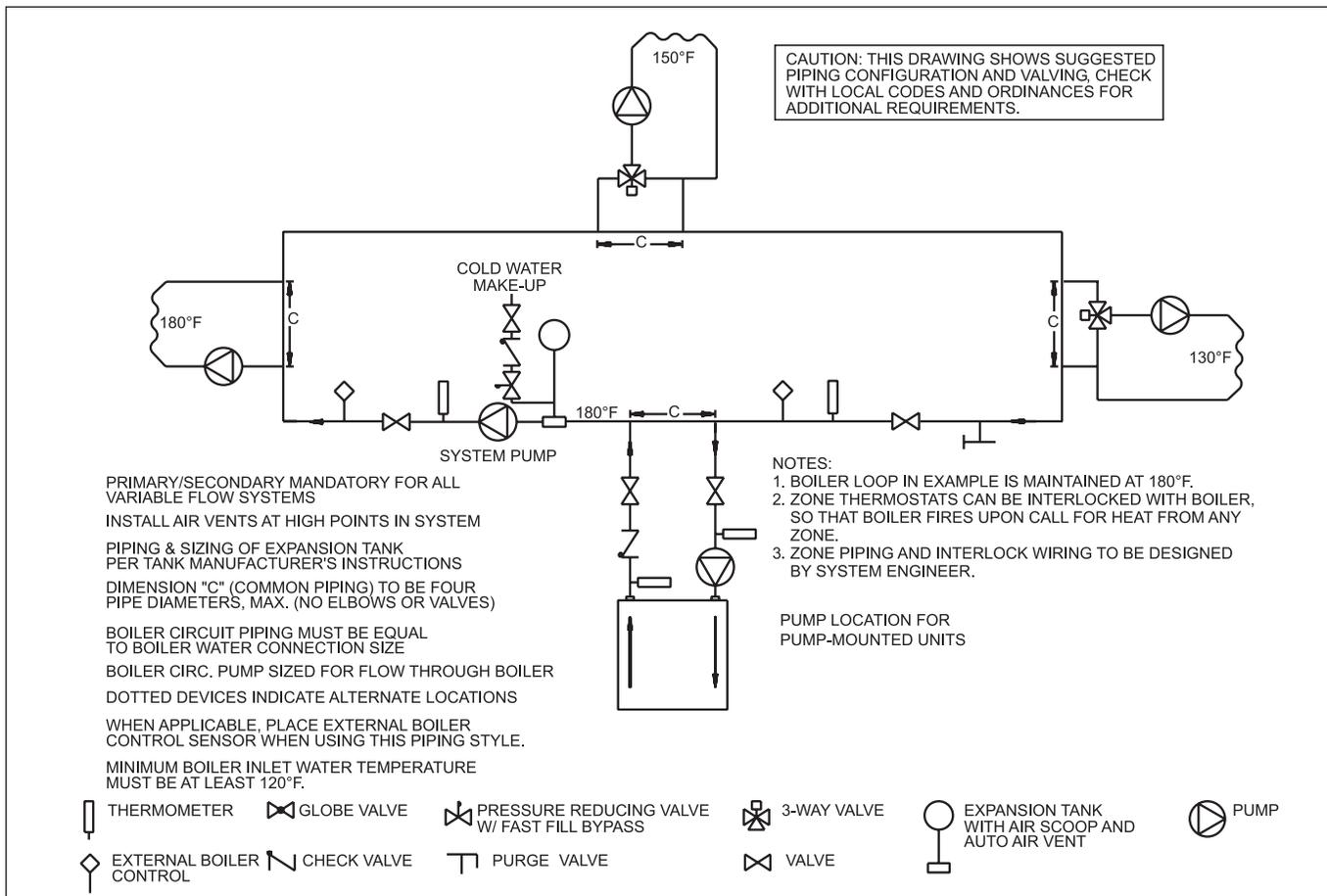
Figure 6. Hydraulic Piping — One Boiler, Multi-Temperature System.
