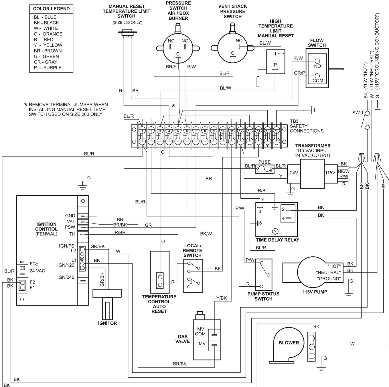
Figure 15. Wiring Diagram, ON/OFF Boiler or Water Heater.
