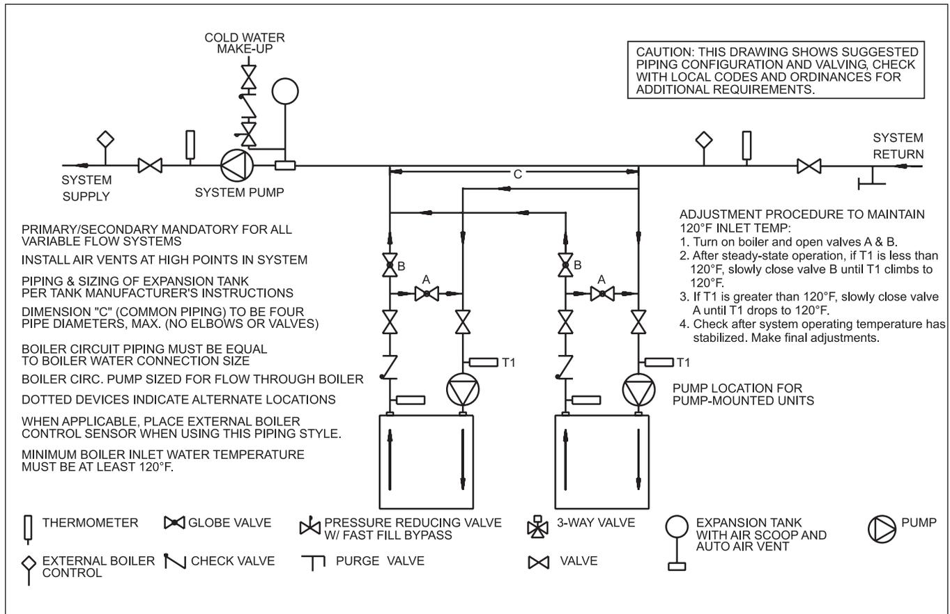
Figure 8. Hydronic Piping — Primary-Secondary, Reverse-Return, Low Temperature.
