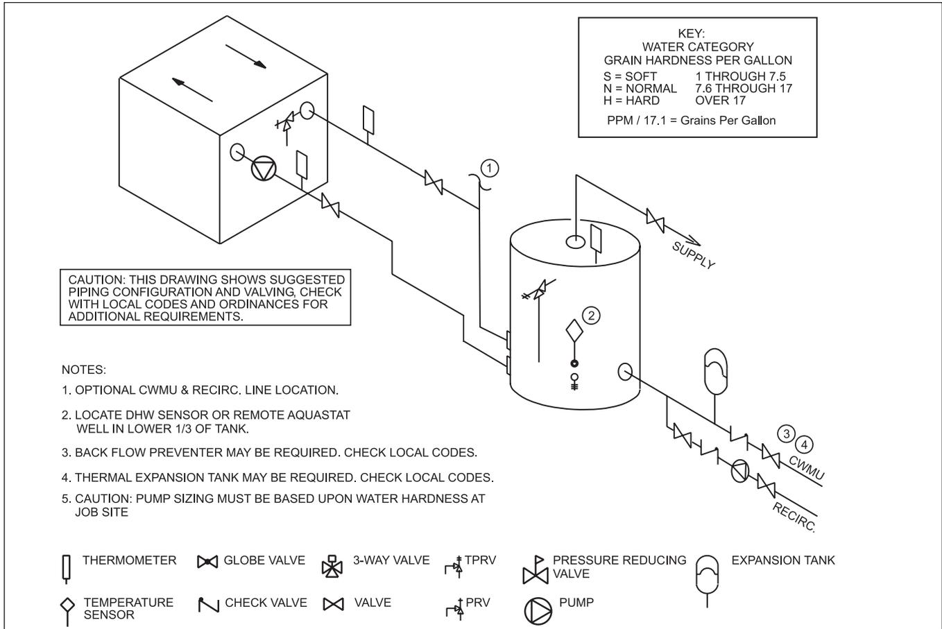
Figure 9. Water Heater Piping — One Heater, One Tank.
