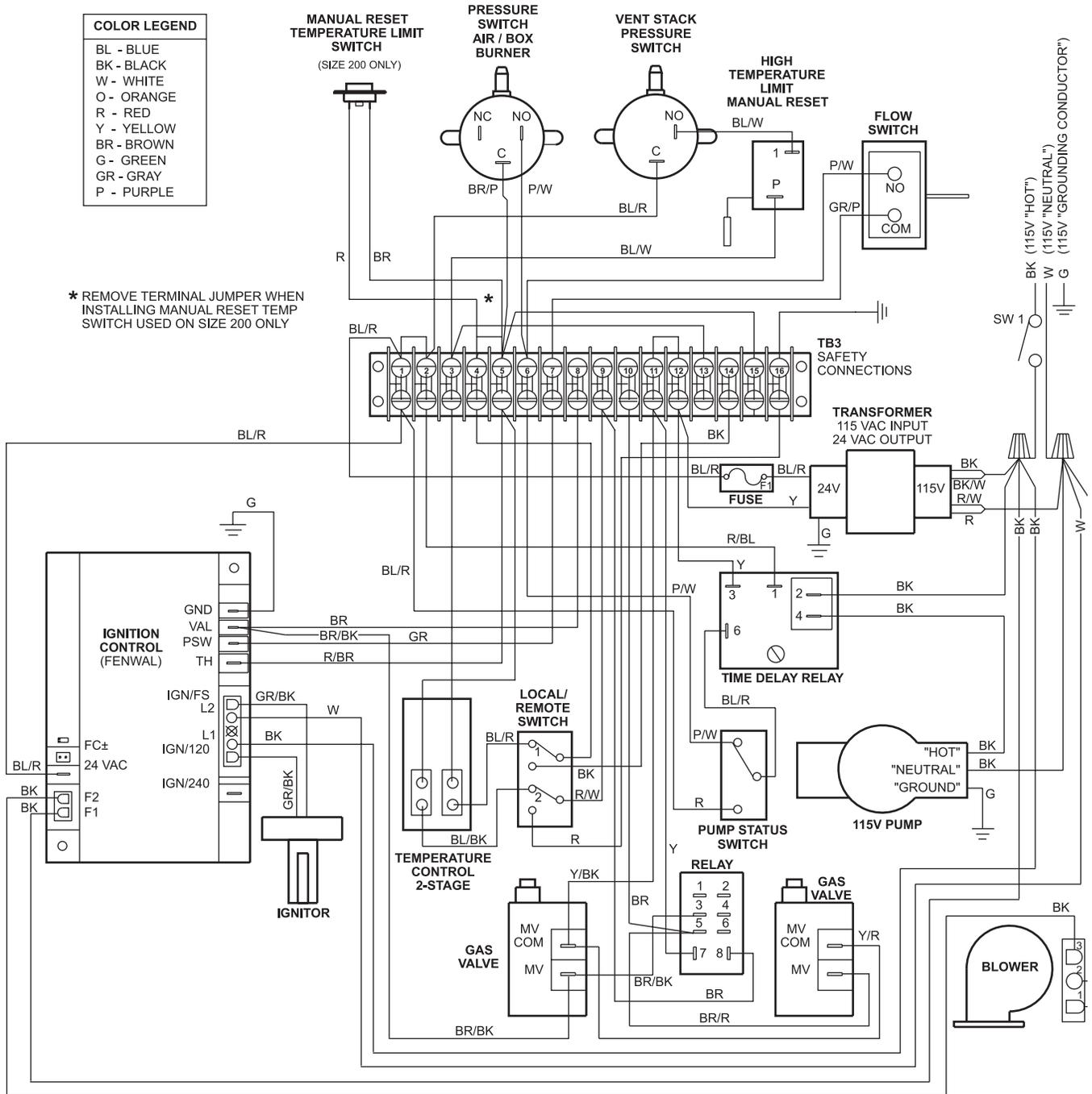
Figure 16. Wiring Diagram, 2-STAGE Boiler or Water Heater
