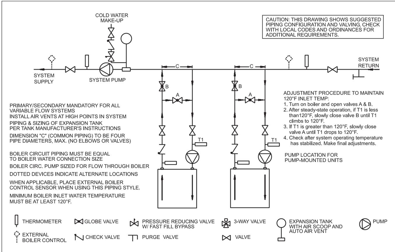
Figure 5. Hydraulic Piping — Multiple Boilers, Low Temperature System.
